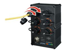
Step 4: Insert the waterproof M12 power connector into the port of the power input.
