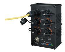
Step 3: Turn clockwise to tighten the screw nut of the waterproof RJ45 connector.
