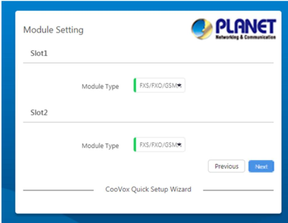
This step is only for IPX-2200 and IPX-2500. If you have installed FXS/FXO/GSM/WCDMA modules on both Slots then just simply click on [Next](#) button to continue. If you have installed E1/T1/BRI modules, please select the module type accordingly. For more configurations please refer to [Module Settings](#).
