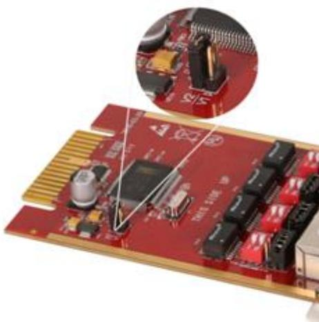
The jumpers shown in the picture below are for crossover cables and straight cables to connect a BRI connection.
