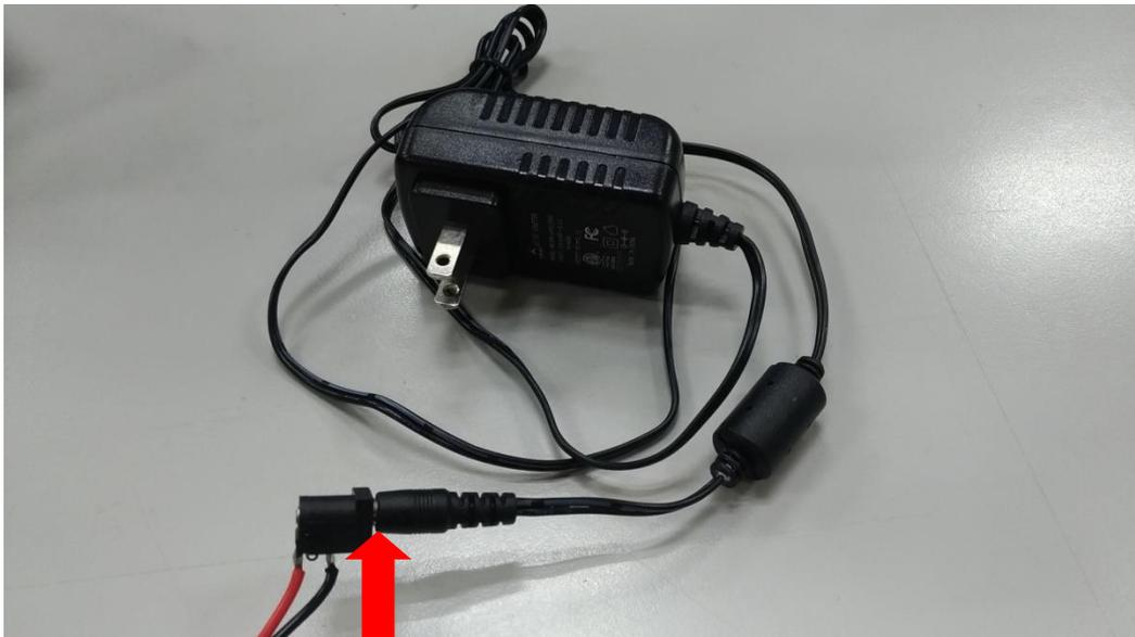
**Figure 2-5:** Connecting Power Cable with Power Adapter
