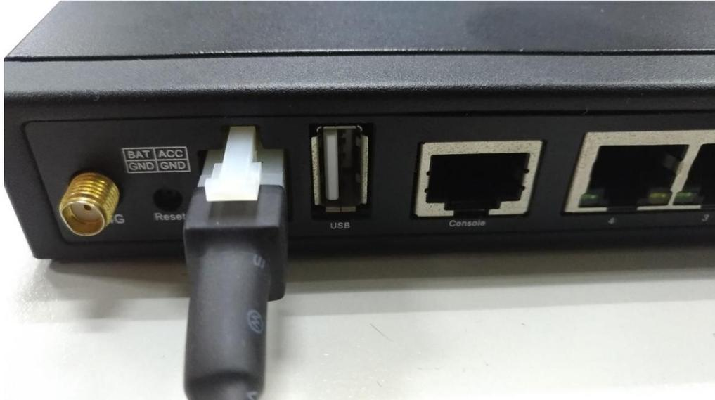
**Figure 2-4:** Plugging in the Power Input
