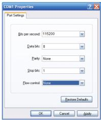
Figure 4-2: COM Port Configuration
