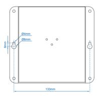
Figure 4-2: Getting mounting holes aligned
