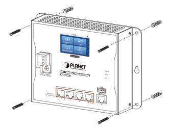
Figure 4-3: Router is screwed to the wall
