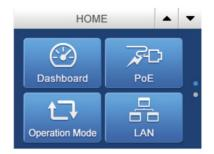
The Settings menu allow user to access different router and PoE features. Tap Up/ Down to access all settings.
