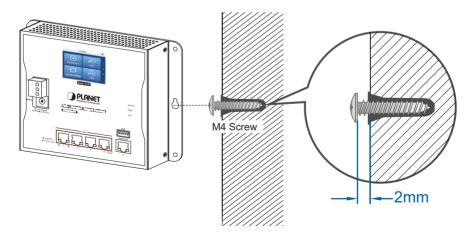
Figure 4-4: Router is hung on the wall
