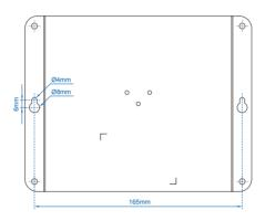
Figure 4-1: Getting mounting holes aligned (WGR-500-4PV/4P)
