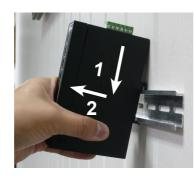
Figure 5-3: Removal of Device from Track
