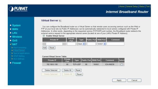
Enter valid ports in the **Virtual Server** section of your router. Please make sure to check the box on this line to enable settings. Then the device can be accessed from WAN by the router's WAN IP address.
