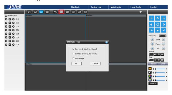
You may select bit rate type you would like to view on your computer. The bit rate type can impact bandwidth consumption on IE.
