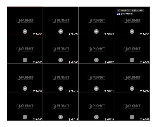
The main/live view is the first interface displayed once you access the HDVR through local display. It displays the live video of all cameras added to the HDVR and the above patterns chosen by the user. The interface has many functions explained below.
