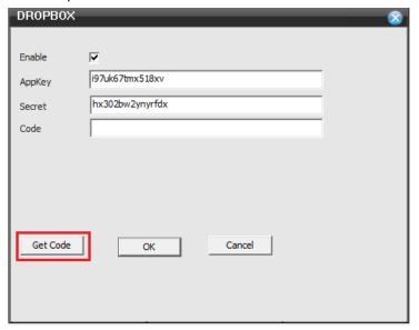
3. In the newly opened page, follow the prompts and finally copy the Code value in the following figure to the "Code" column in the "Network Service→ Dropbox" configuration interface.
