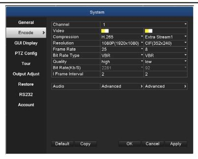
Picture 5.14 Hybrid/ Analog Encode Setup
