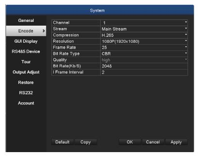
Picture 5.13 Digital Encode Setup
