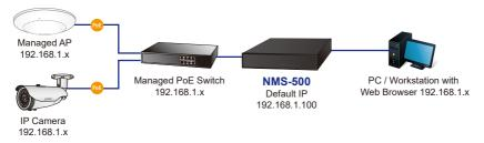
**Step 2. Switch/Router:** Log in to the Switch's Web User Interface and **enable** the **SNMP, LLDP and NMS controller** functions.
