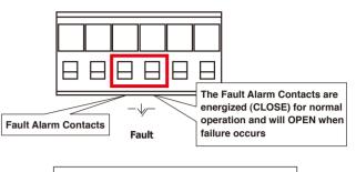
Insert the wires into the fault alarm contacts
