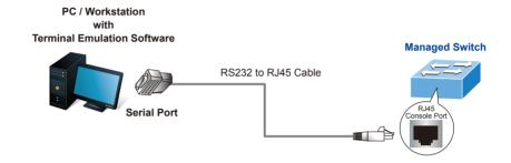
Figure 3-1: Managed Switch Console Connectivity
