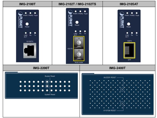
Figure 2-1-2: Reset Button of Modbus Gateways
