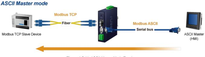
Figure 4-5-11: ASCII Master Mode Topology
