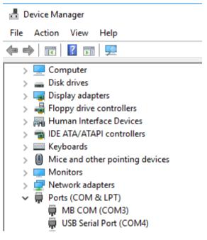
Figure 5-3-4 : Virtual COM Ports
