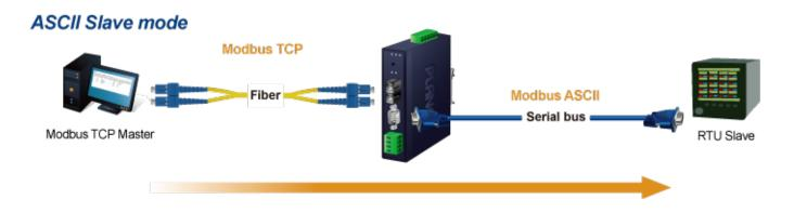
Figure 4-5-9: ASCII Slave Mode Topology
