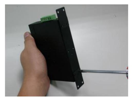
Step 3: Use the screwdriver to screw the wall-mount plate on the Modbus Gateway.
