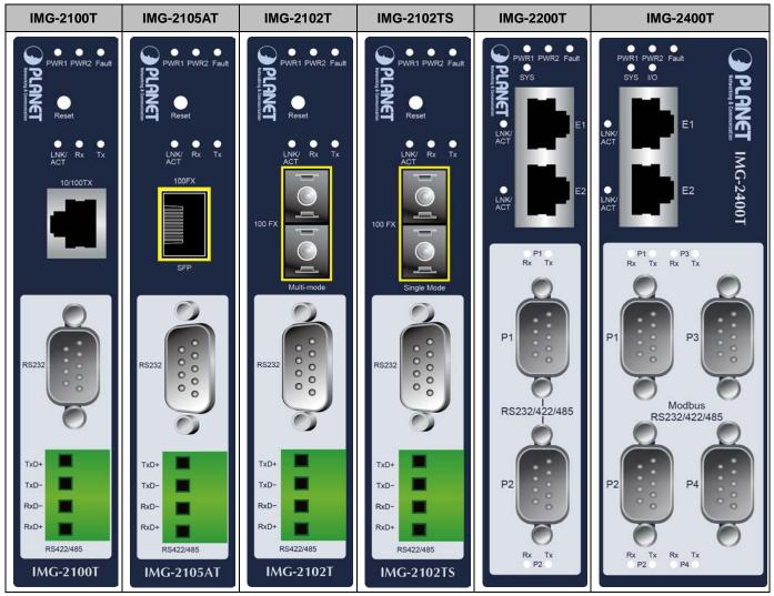
Figure 2-1-1: Front Panels of Modbus Gateways
