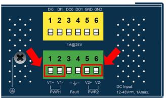
Figure 2-1-5 IMG-2400T Upper Panel
