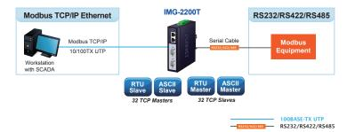
The advantage of having the IMG-2X00T Series is to assist users to build an industrial environment between the Modbus TCP/IP Protocol and the Modbus RTU/ ASCII Protocol easily, thus offering an application solution to the industrial control equipment without Ethernet ports and the industrial control equipment can only control through an industrial PC workstation or industrial control panel. Supports extensive LED indicators for network diagnosis
