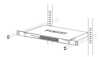
Figure 6: Mounting the Gigabit Ethernet Switch in a Rack
