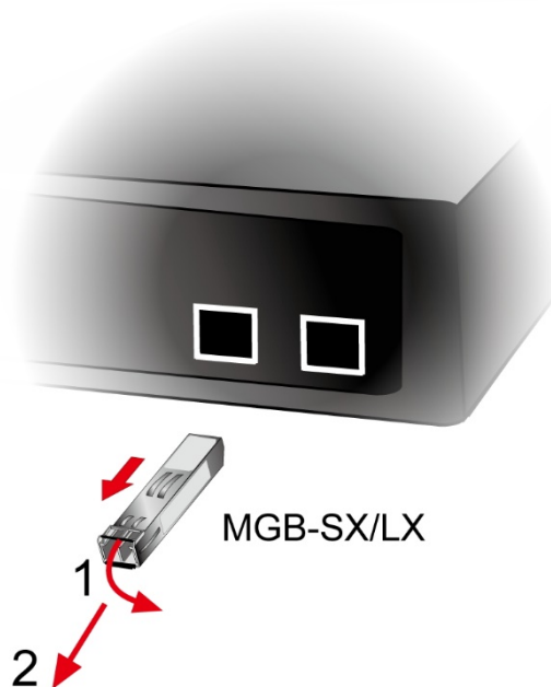
Figure 2-2-5: How to Pull Out the SFP/SFP+ Transceiver
