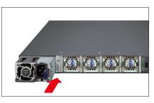
Figure 3-3 Tightening the Thumbscrews
