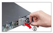
Figure 4-1 Removing the Power Supply Unit
