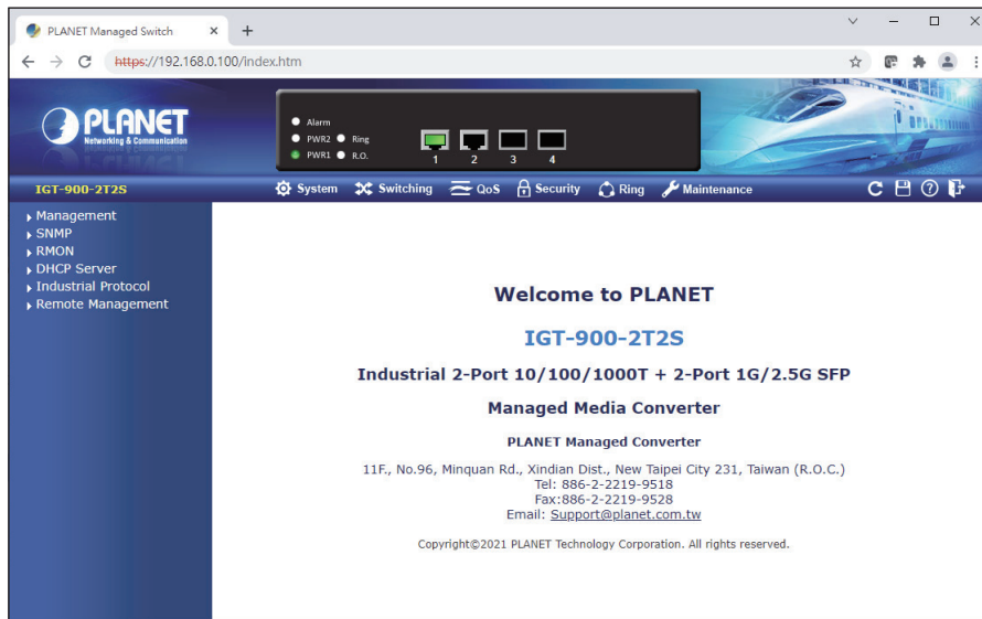
Figure 4-4: Web Main Screen of Industrial Managed Media Converter
