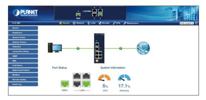
Figure 4-3: Web-based Main Screen of LoRaWAN Gateway
