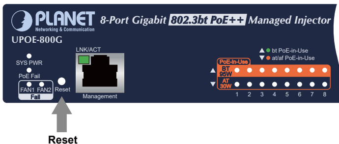
Figure 4-1: 802.3bt PoE++ Managed Injector Hub Reset Button
