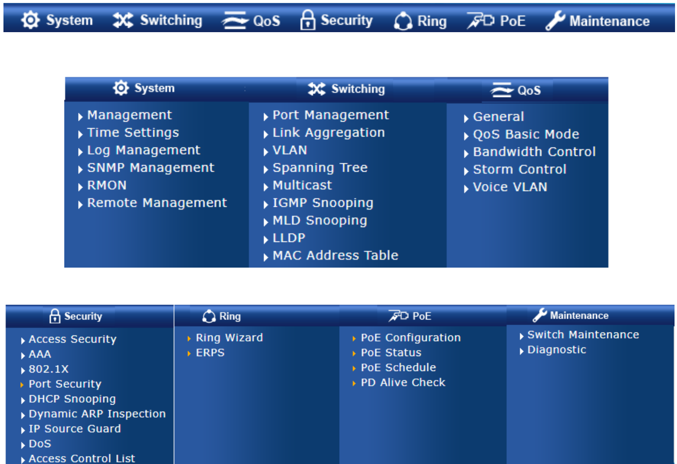
Figure 4-1-2 Managed Switch Main Functions Menu
