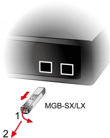
Figure 2-1-8 How to Pull Out the SFP Transceiver
