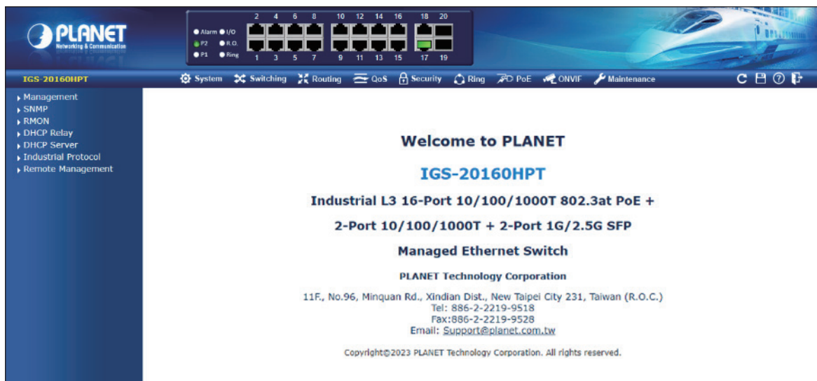
Figure 5-6: Web Main Screen of Industrial Managed PoE+ Switch
