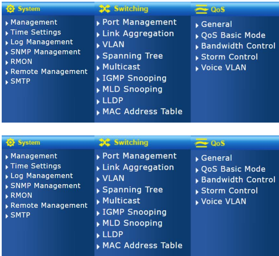
Figure 4-1-2: Managed Switch Main Functions Menu
